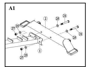
Attach Rear Stabilizer (2) to the Main Frame (1) using two 1/2" X 4" Hex Bolts (21), four 1/2" Washers (25), and two 1/2" Nylon Nuts (27). Tighten bolts.
